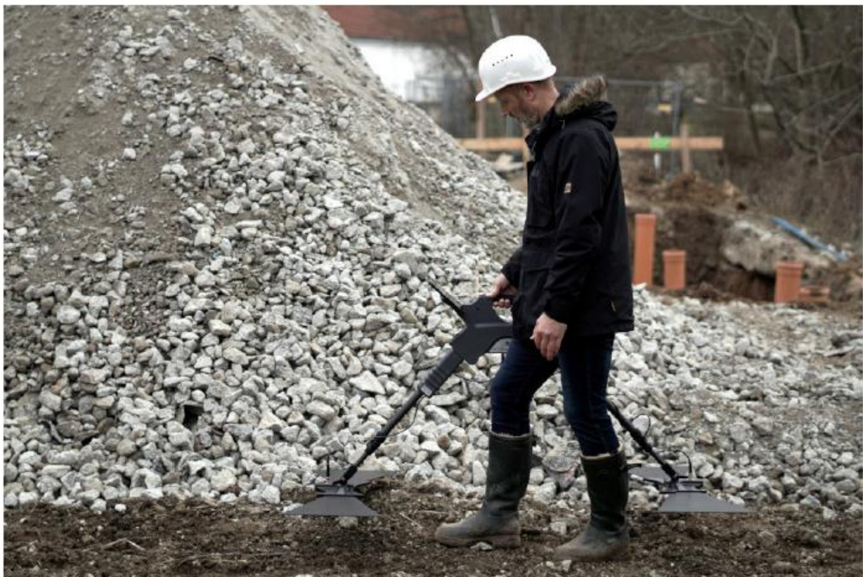
Figure 6.1: Holding the Gepard GPR before starting the scan
