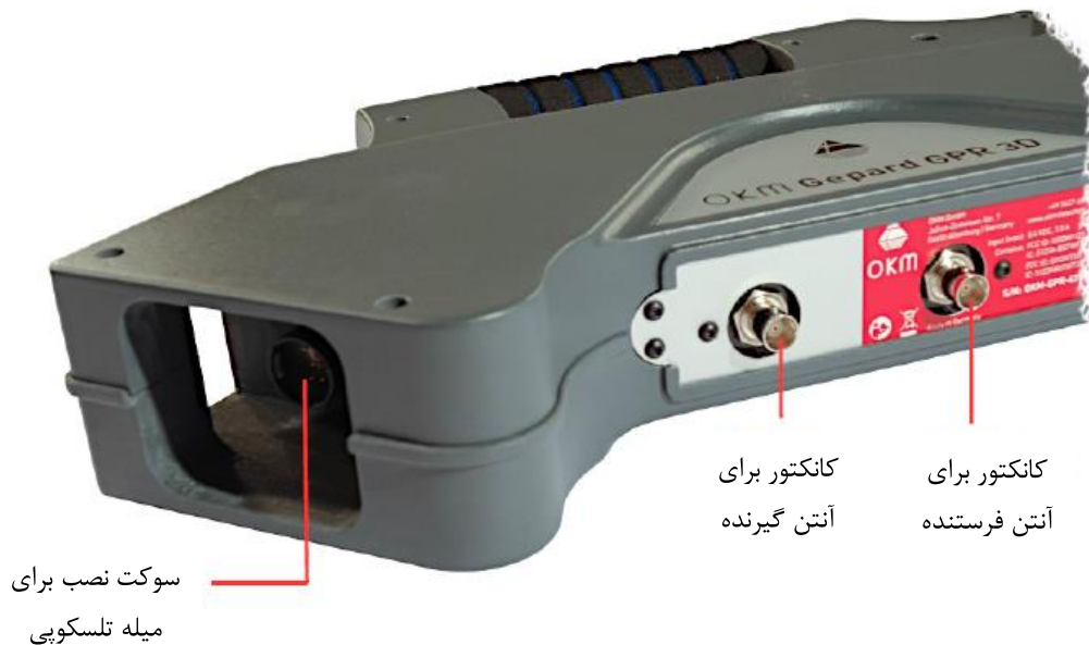
Figure 4.2: Connector panel of the control unit
