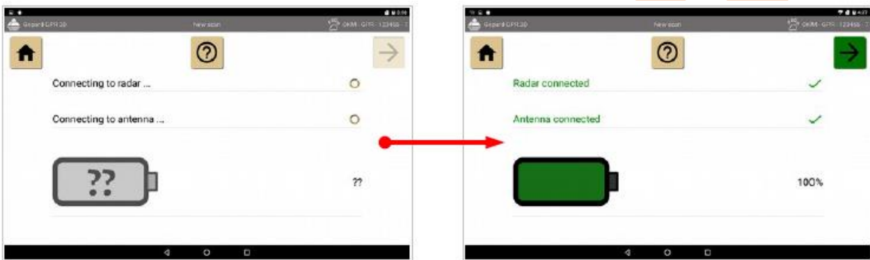
Figure 7.7: New Scan - Establish WiFi connection
