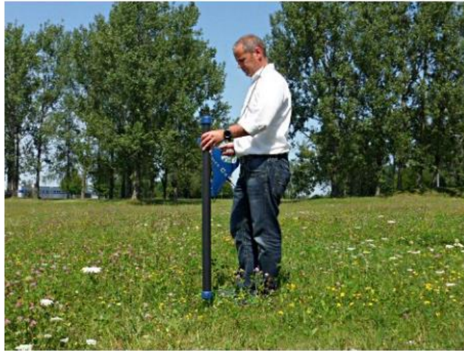
Figure 7.4: Position of the Super Sensor during a measurement
