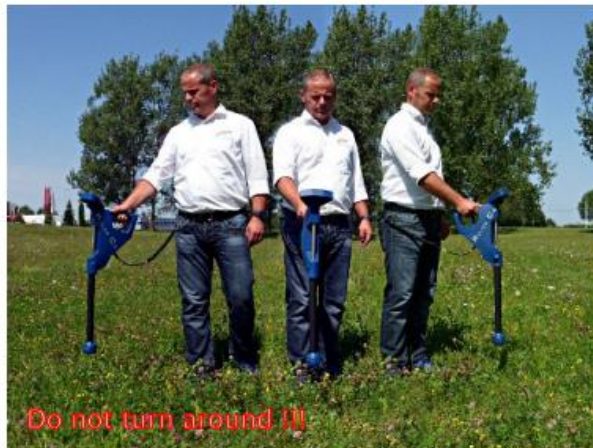
Figure 7.10: Pivoting or turning of the probe falsifies the measurement
