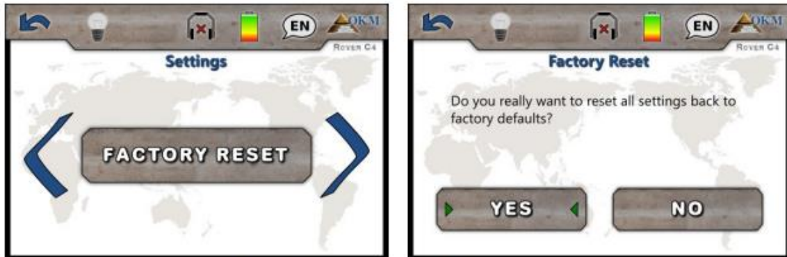
Figure 7.25: Settings – Reset to factory defaults
