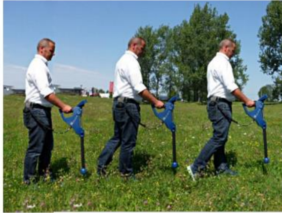
Figure 7.9: Probe should point always to the down and should not be turned
