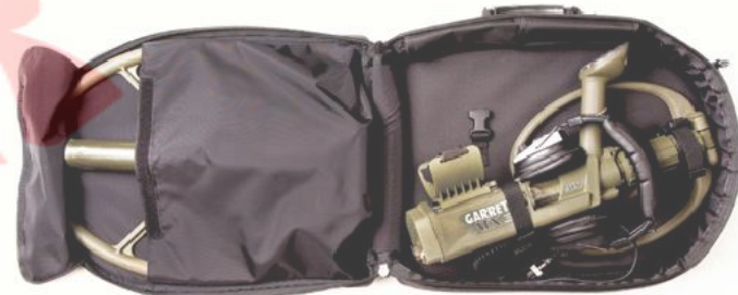
Figure 2: ATX with DD coil attached + Deepseeker coil + headphones. close velcro flap to secure Deepseeker coil.❖Note
