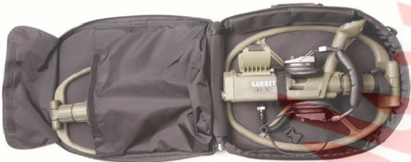
Figure 5: ATX with Deepseeker coil attached + DD coil + headphones. close velcro flap to secure DD coil. Note
