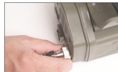
Hand-tighten connector collar.
